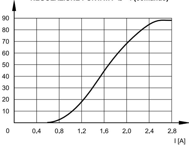
**Q [l/min] REGOLAZIONE PORTATA Q = f (pB)**
