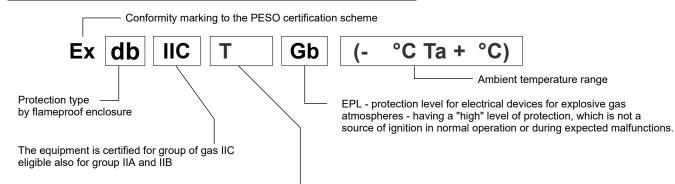
Temperature class/max surface temperature see par. 4.3 -
