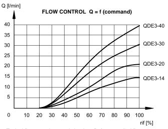
Typical flow rate characteristics A  $\rightarrow$  B for controlled flow rate 14 - 20 - 30 - 40 l/min as function of the command signal.
