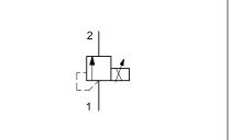
**NOTE**: The maximum operating pressure is the sum of set pressure and return flow pressure.
