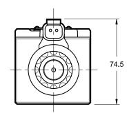
connection for DEUTSCH DT06-2S male connector code **WK7** (W7 version only) code **WK7D** (W7 version only - coil with diode)
