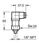
This indicator is a pressure switch sensitive to the filter input pressure, which switches an electrical contact when the filter element has reached the clogging limit
