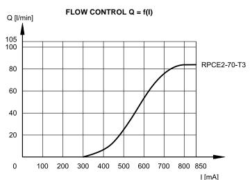
Typical flow control curves for flow rate  $E{ o}T$ , according to the current supplied to the solenoid.
