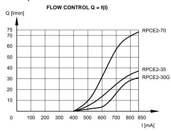
Typical flow control curves for flow rate  $E \rightarrow U$  according to the current supplied to the solenoid.
