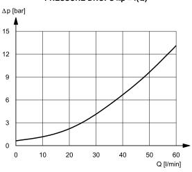
Pressure drops with free flow  $U \to E$  through check valve.
