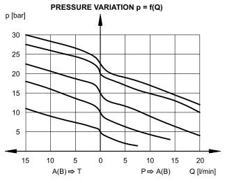
The curves have been obtained with inlet pressure 100 bar.
