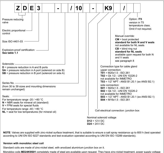
Monobloc coils **MD24K9S01** completely made of steel are available upon request. They have zinc-nickel treatment, power supply voltage D24 and cable gland connection type S01. Other variants for voltage and cable gland connection are available, always on request.
