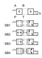
Type **TB**: 1 solenoid side B 2 external positions with return spring
