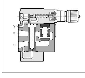
The Z\*-P type valves are used when a branch with a lower pressure than the main one is desired in the hydraulic circuits.
