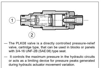
— The circuit pressure acts on the shutter which is directly loaded by a spring on the opposite side. Once the set pressure is reached, the shutter opens, and discharges the excess flow in port 2 connected directly to the reservoir.
