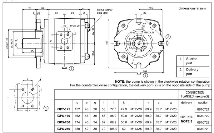
**NOTE 5**: For applications with delivery pressure > 200 bar, a special connection flange cod. 0610725 is required.
