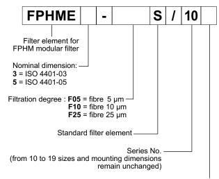
N = NBR seals for mineral oils (standard)V = FPM seals for special fluids (upon request)
