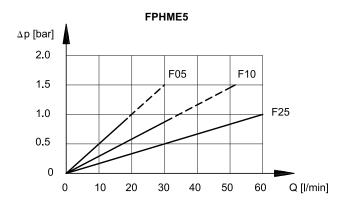
NOTE 2: The filter size has to be selected so that with nominal flow rate, the total pressure drop is less than 1.2 bar.
